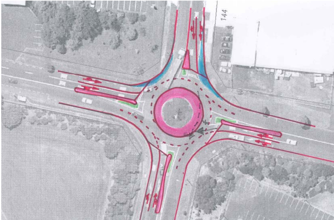
Figure 9.3: Sketch showing a C-Roundabout configuration. The shaded areas depict kerb cutback (shown blue), existing islands to be removed (shown green), and new traffic islands (shown pink).
