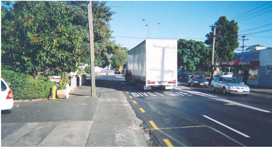
Figure 7.1 Semi-trailer straddling both entry lanes while entering the Frost Road / Carr Road roundabout from the Carr Road approach.
