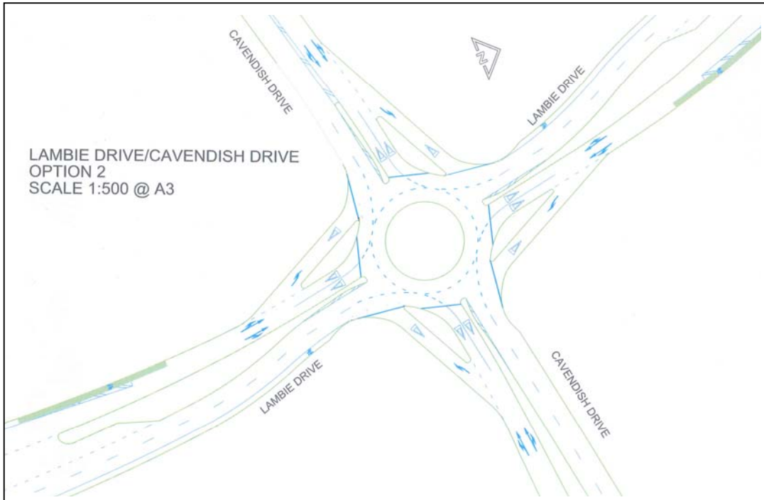
Figure 8.2 A C-Roundabout option in Manukau City, Auckland, that includes left-turn slip-lanes for additional roundabout capacity (central island diameter is 20 metres as in Figure 8.1). Note the Lambie Drive approaches are dual-lane and are shown with merge areas upstream of roundabout entries.
